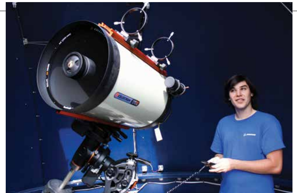
Tyler Ram operates the robotic controls on the 14-inch Schmidt-Cassegrain telescope installed in the Gira Center observatory.
